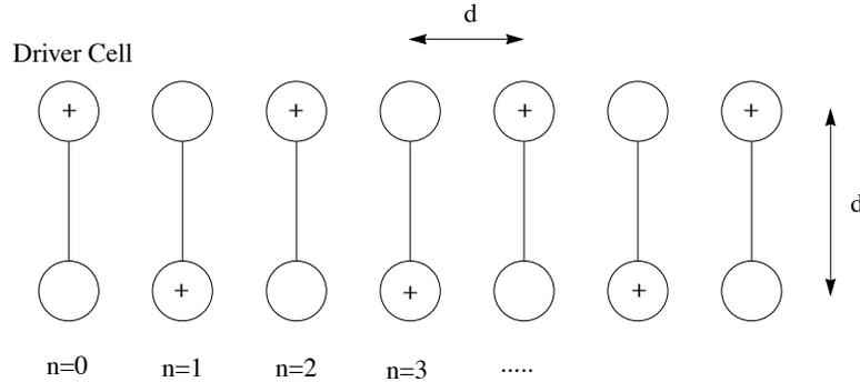
Each cell has one excess electron that can move relatively easily between a pair of metal atoms. There is a single “driver” cell on the left side of the chip that we can force into the “+” state, i.e. the electron is on the upper metal atom. Since we now are experts at the Ising model, we will denote the state of the  $i^{\text{th}}$  cell as  $S_i$ . This variable tells us where the electron is in that cell. In the above diagram, we have  $S_1 = -1$  and  $S_2 = +1$ .
